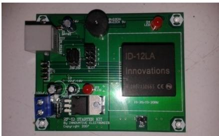
Gambar 1. Rfid (Radio frequency Identification)
