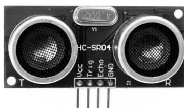
Gambar 5. Sensor Ultrasonic
