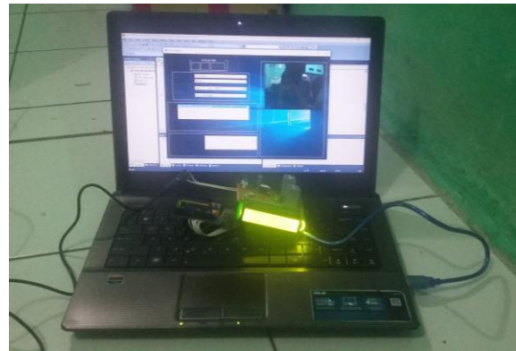
Gambar 8. Tampilan Alat Prototype Absensi Berbasis Face Recognition
