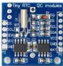
Gambar 5. RTC DS-1306 (sumber : http://elty.pl )
