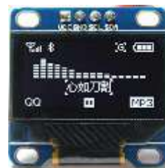
Gambar 7. I2C 128x64 OLED (sumber : http://amazon.com )
